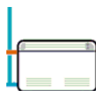
Figure 8. Fancoil units connected to the network
